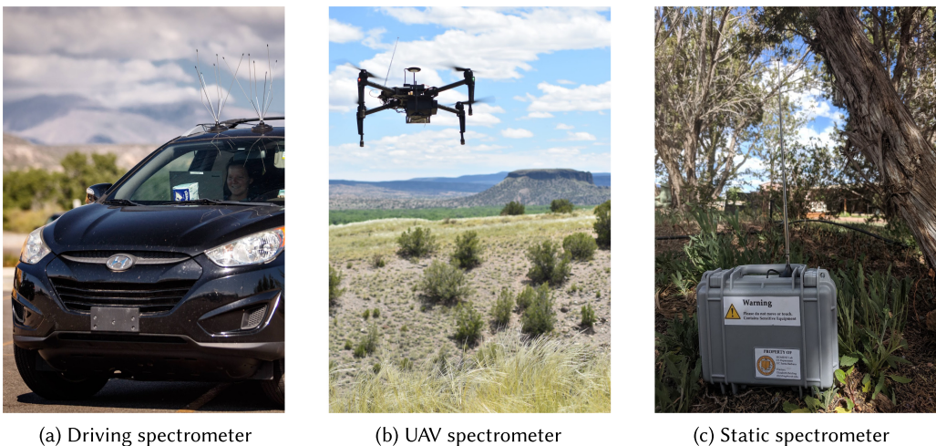
Fig. 5. Different spectrum measurement methodologies used to measure TVWS spectrum availability.
