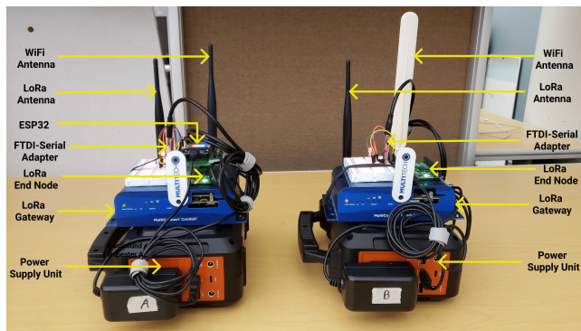
Figure 5: Implementation of LoRaX compound repeaters.
